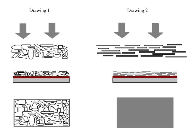
As shown by the arrows, contaminants attacking each film could move easily through the porous surface of the conventional coating while those same contaminants would have a more difficult time working their way through the much tighter stainless film.
